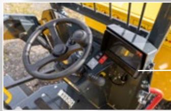
Protected IP67 rated 7" LCD Monitor
