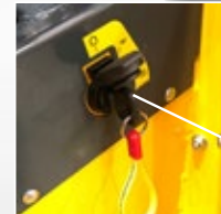
Two stage start inhibitor safety system
