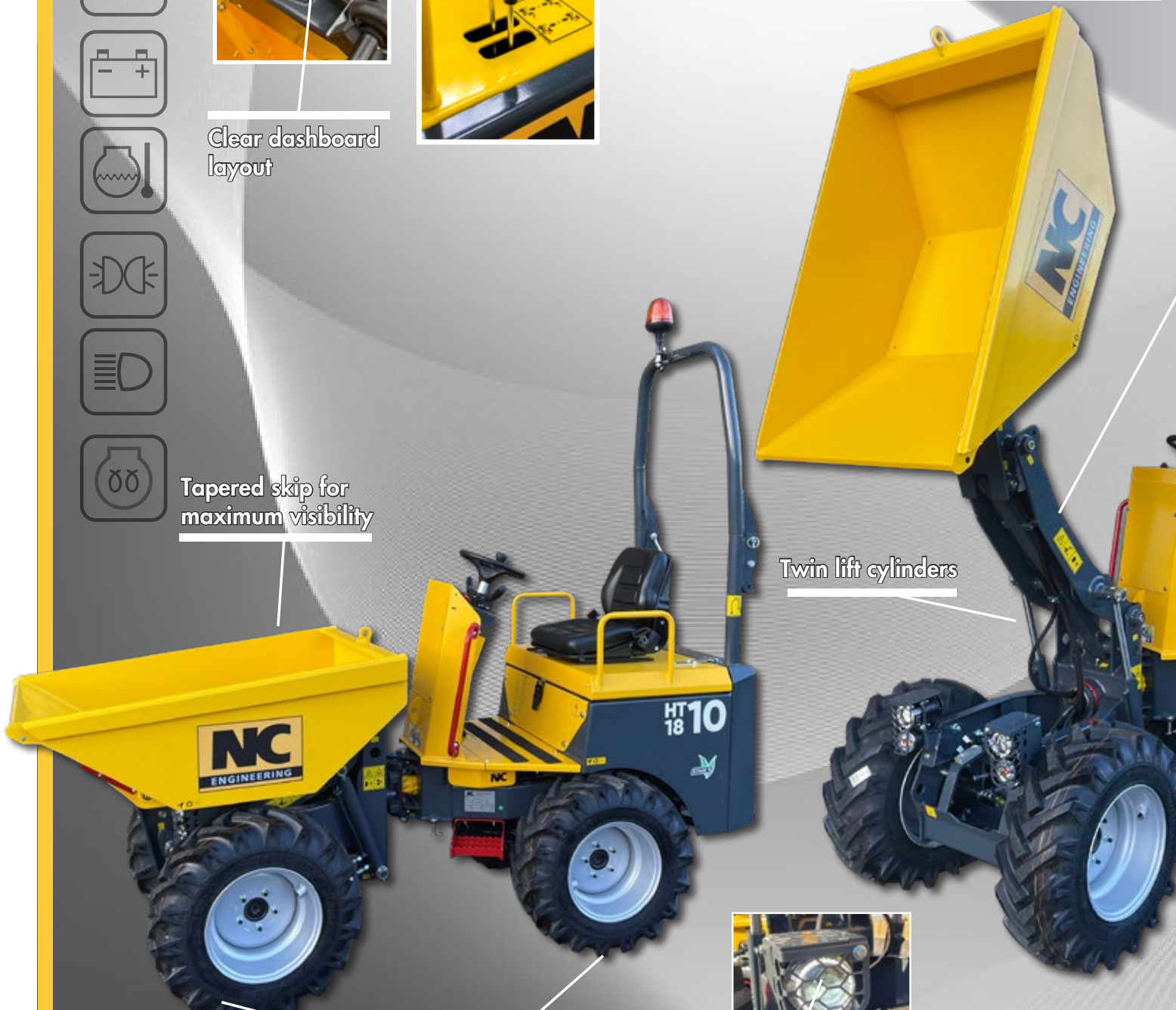
Four wheel drive Twinlock system
